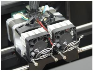
4. Carefully pull the screws out and please make sure that you do not loose any parts. The black plastic spacer comes loose after the bolts are removed. Place all removed parts besides the printer. Manually place the cooling fans towards the back so they are out of the way, keep a track which one is for the right and left side by adding a sticker or something.
