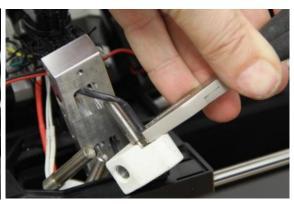
25. Place the cold block assembly onto the carriage. And carefully guide the thermocouple cables into the milled groove of the cold-block so it will not be pinched by the extruders.
