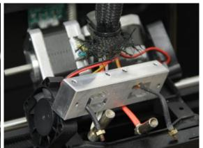
13. Guide the thermocouple sensors gently out of the cold-block, if it is too tight you can bend the tab that holds the hotend so it will create more room for the thermocouple sensor to slide out of the block.
