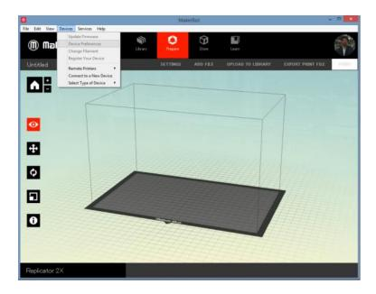
Since the gear diameter is smaller on the Bondtech kit the c-c distance between the nozzles is also bigger than original. In the dialogue box change the value for Toolhead Offset Settings from 35000 um to 38500 um
