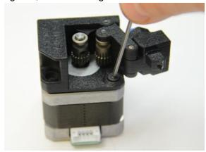
20. Insert the M3x8 Socket head bolt into the other hole of the extruderbody, tighten but do not overtighten.
