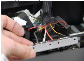
24. Thread the thermocouple into the heatblock by turning the heatblock, NOT the thermocouple. Finish off by tightening the thermocouple onto the block with a plier or similar.
