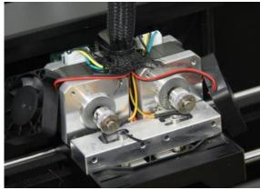
6. Loosen the set-screw holding the extruder gear onto the motor shaft and remove the gear.
