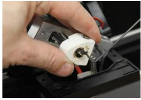
11. Untighten the thermocouple from the heatblock just so it can move, DO NOT TURN IT MORE THAN ½ TURN!
