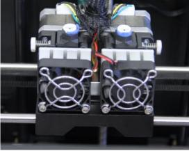
29. Remove the blue plastic clip from the pushfit connector and push the guide tube into the connector, when the guide tube is in place refit the blue plastic clip.
