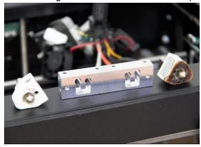
23. Start by guiding the thermocouples gently through the coldblock, please not the orientation of the coldblock. In the new coldblock there is enough room for the thermocouple to easily pass through the coldblock.
