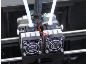
30. The new BTI/Bondtech cold block makes it possible to adjust the height of the hotends from the outside making it much easier than the original coldblock that required a disassembly in order to adjust the nozzle height. The hotend is held securely in place by a set-screw that presses a tab that clamps the hotend.
