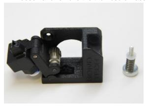
18. Place the extruder onto the motor oriented like the photo.
