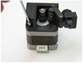
21. Align the primary gear with the secondary gear and tighten the setscrew.
