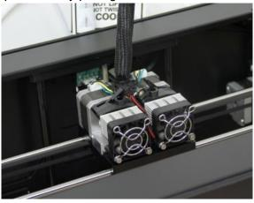
3. Loosen the front M3 bolts holding the fan protector, heatsink and motors together
