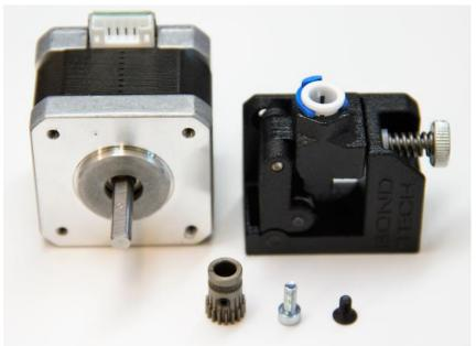
16. Start with installing the primary gear onto the shaft of the steppermotor.
