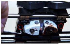
27. Place the motors with the extruders onto the carriage and align it with the coldblock assembly.
