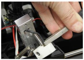
12. Rotate the heatblock with the heatbreak around the thermocouple carefully so it is fully loose. Repeat this for both hotends.
