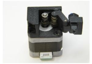
19. Insert the countersunk M3x8 screw in the countersunk hole of the extruderbody and tighten, do not overtighten!
