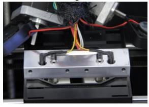
26. Remount the M3 screws from the bottom of the carriage securing the cold block.
