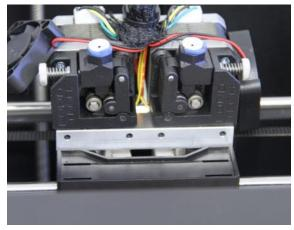
28. Remount the fan guide, fan, spacers and heatsink with the bolts.
