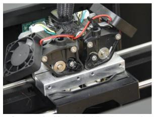
5. Remove the M3 bolts holding the extruder assembly onto the motors and remove the parts
